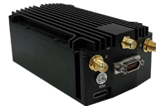
11.7×6.2×3.8cm/349g 11.7×6.2×4.2cm/360g 1Watts×2/2Watts×2 Extended WIFI/HDMI/SDI (Air to G. 20~50/50~100KM)
